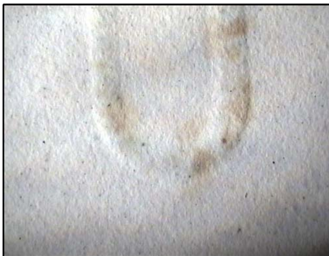
Fig. 10 Optical micrograph of a sample consisting of: bronze as support insulated by alumina (150 \mu\text{m} ), Ni20Cr heating trip and alumina top coating. Stains on the metal strip were observed after an accelerated corrosion test and found to be due to iron contamination of the sprayed heating element
