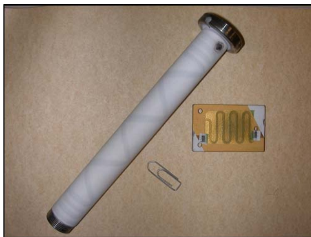
Fig. 11 Two types of heaters successfully implemented: a runner nozzle for polymer injection molding apparatus as described in the patent publication (Ref 8) and a heating plate
