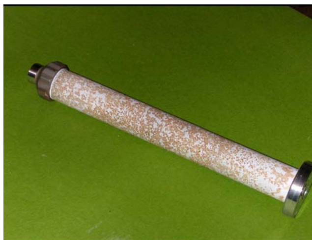
Fig. 2 Stains on the first alumina layer sprayed on sand-blasted nozzle left at room temperature in humid environment
